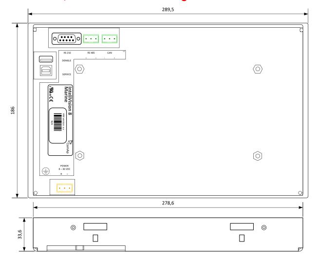
Note: Measurements are in millimeters
