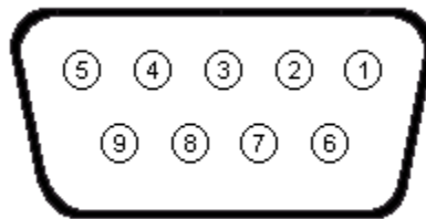
Figure 4-5. MODBUS Communication Port Terminal Positions
