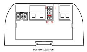
To activate Power supply mode connect pin 7 and 8.
