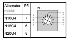
P5 [kVA] limits the maximum excitation voltage of the alternator and therefore the maximum output power of the generator. This parameter is an integral over time, allowing a 200%-300% overload for a few seconds without limiting and illuminating L2 (Red LED blinking 3 times) or a slight overload for a longer period.
